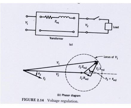
$V_{1} = V_{2} \angle 0^{0} + I_{2} \angle \theta_{2}^{0} Z_{eq1} \angle \theta_{eq1}^{0}$ Clearly  $V_{1}$  is max imum when  $\theta_{2} + \theta_{eq1} = 0$ ; or  $\theta_{2} = -\theta_{eq1}$
